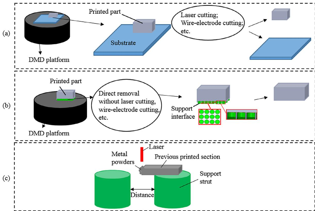
Fig. 1. (a) Conventional process of removing printed parts; (b) schematic of proposed support interface method and (c) illustration of printable distance.
