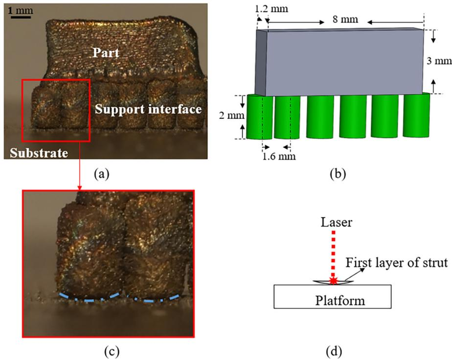
Fig. 3. (a) Printed part; (b) design and dimensions of the support interface and test part; (c) close view of the connection between the struts and substrate; and (d) schematic of laser energy distribution.
