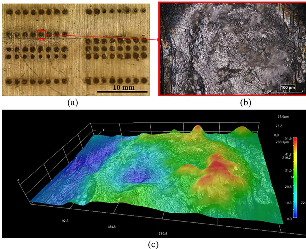
Fig. 4. Photos of (a) the substrate surface after part removal, (b) the enlarged view of the remaining strut base and (c) micro-surface analysis.
