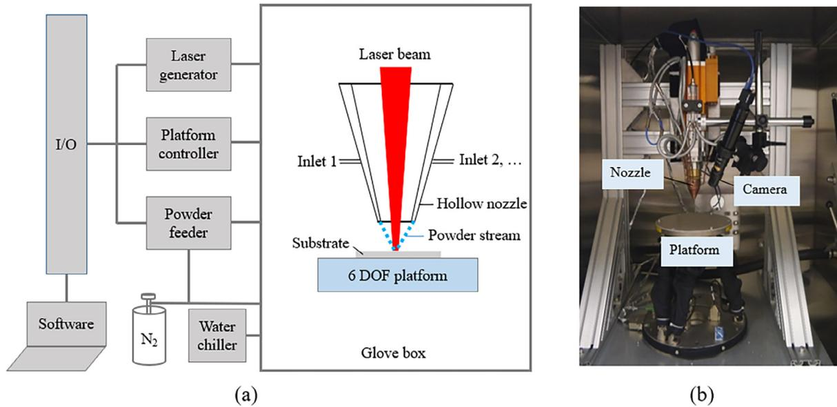
Fig. 2. (a) Schematic of the DED equipment and (b) printer assembly in the working chamber.
